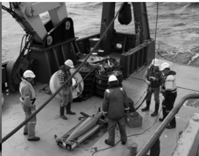
The Australian Integrated Marine Observing System (IMOS) celebrated the first successful deployment and retrieval of a Seaglider in the Southern Ocean. The observations from Seagliders provide data to help researchers understand currents and ocean parameters such as temperature and salinity in the Southern Ocean. Photo by Eric Schulz.
