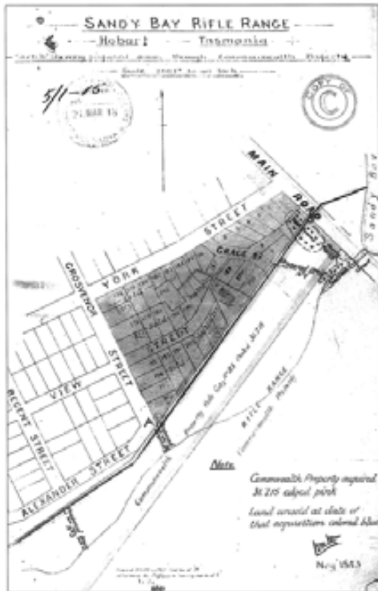
Figure 25: Drainage plan of the arrangement to pipe water from the Golf Links Estate sub-division to the creek and for additional land to be added to the Rifle Range. The plan is useful in showing the creek line and swampy ground. The current University boundary follows the heavy line but includes the lot fronting Sandy Bay Road marked as swamp. Grace Street now extends into the campus Site. The former Golf Club House remains as a residence on lot 270.
