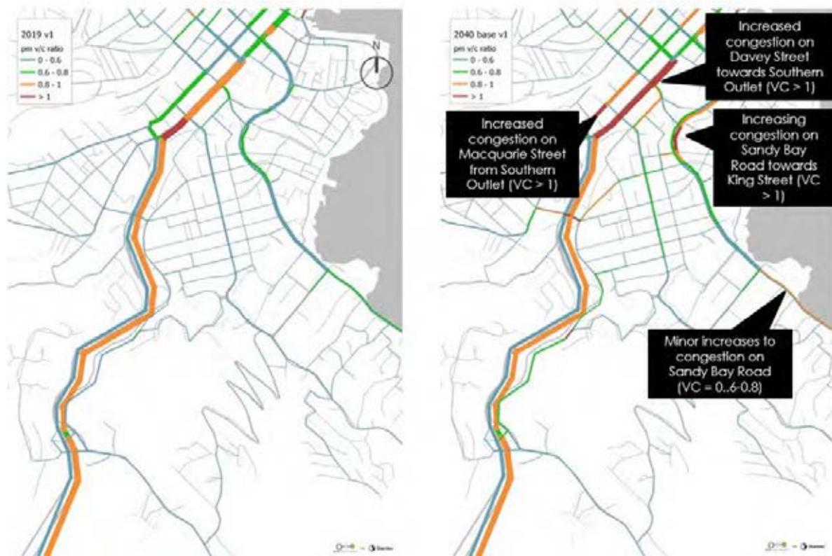
Figure 6.6: Average VC Plots for 2019 Existing Conditions vs 2040 Base Case – 4-6 PM
