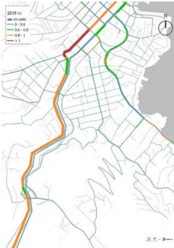
Figure 2.8: Existing Road Network Performance – VC Ratio – AM Peak Period
