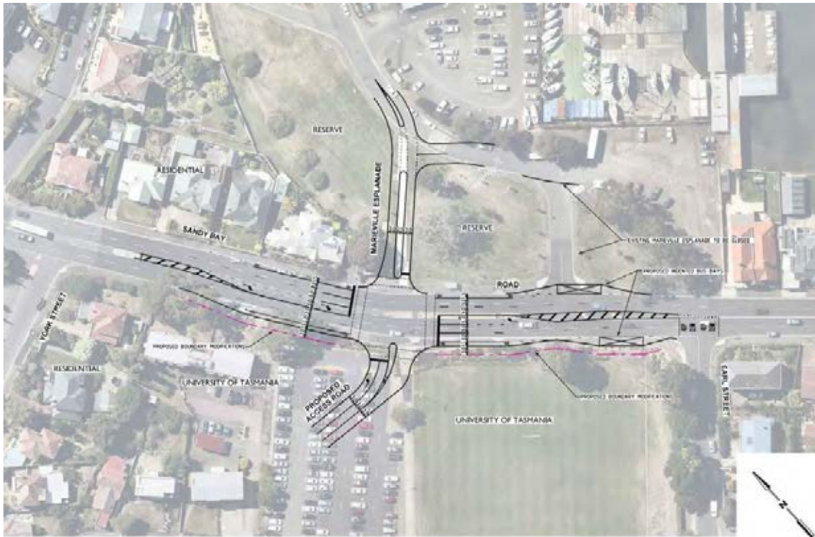
Figure 4.6: Sandy Bay Road Vehicle Access Arrangements – Concept Functional Layout Plan
