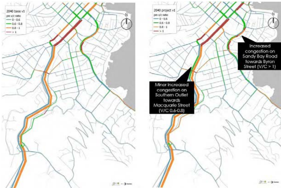
Figure 6.8: Average VC Plots for 2040 Base Case vs 2040 Project Case – 4-6 PM
