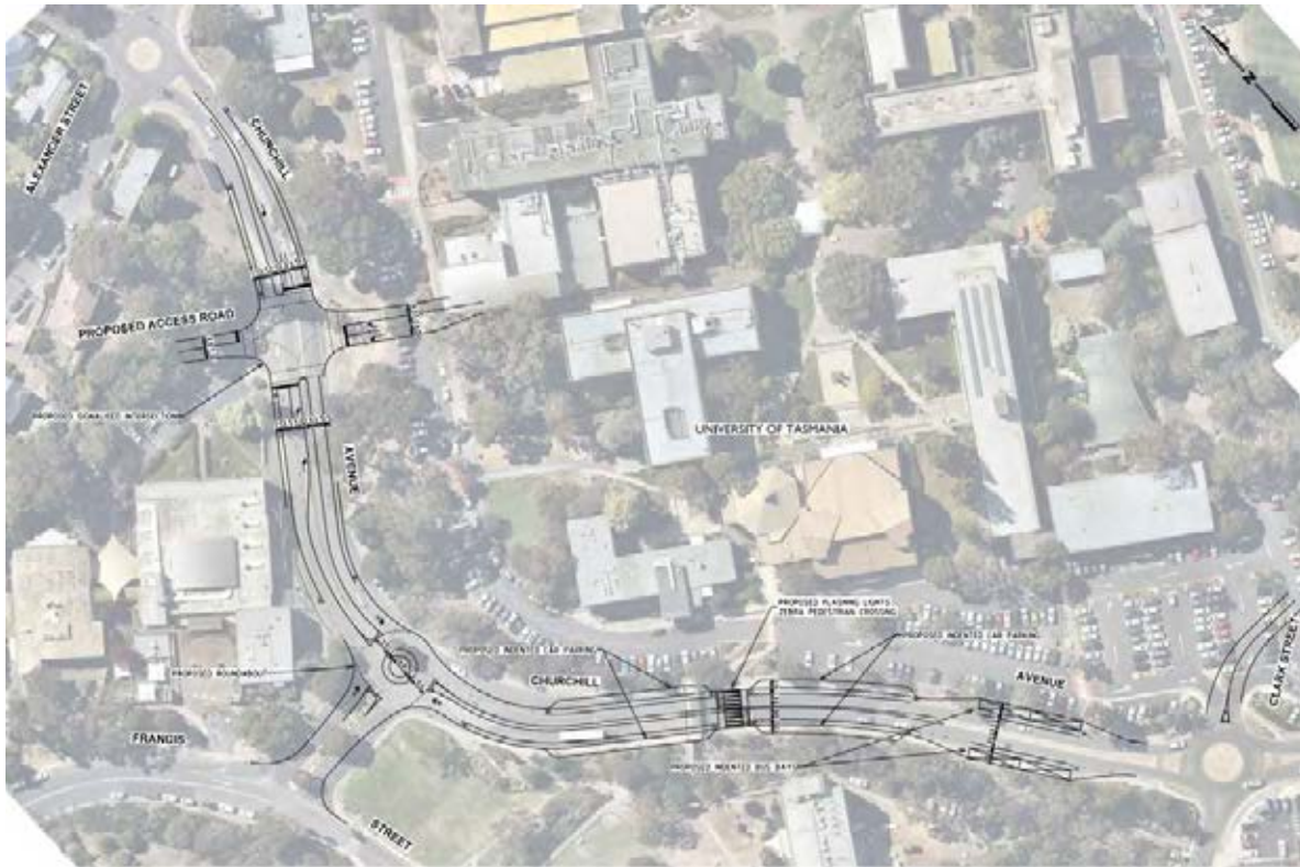
Figure 4.7: Churchill Avenue Vehicle Access Arrangements – Concept Functional Layout Plan
