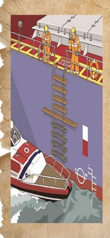
A pilot ladder is used to get on and off ships when at sea. You can see one on the wall next to you.
